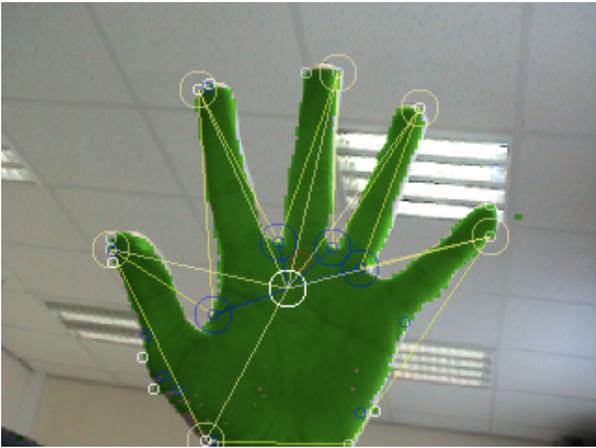
Figure 1. A hand tracking software analysing a hand shape
